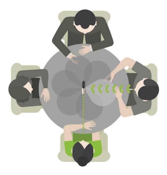
MultiBeam Technology utilizes multiple microphones pointing in six directions, automatically selecting the person who is talking.
