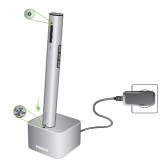
(i) Insert the device into the docking station as indicated. Incorrect insertion may damage the device.
